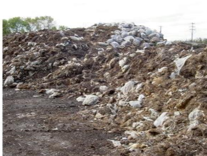
Figure 19. Windrow composting site containing oxo-degradable polyethylene bags in May 2006
