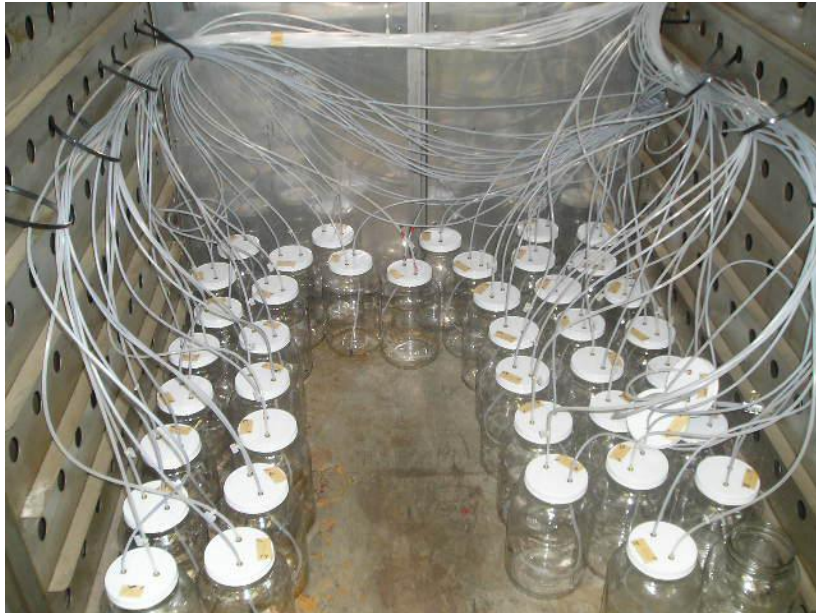
Figure 13. Biodegradation apparatus for testing of biodegradable materials by ASTM D5338.
